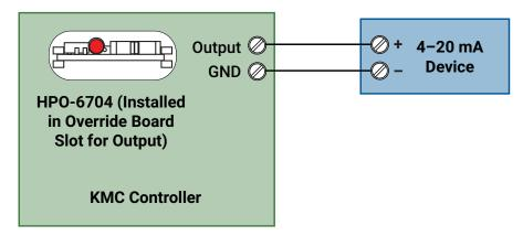
Illustration: HPO-6704 Installed in Compatible KMC Controller
