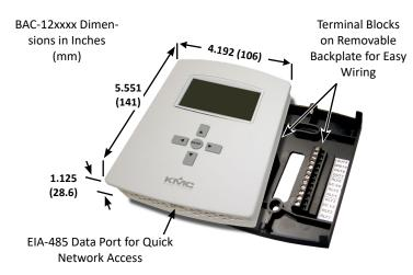
NOTE: Two-piece design allows field rough-in and termination of field wiring to the backplate without needing the FlexStat at the site—permitting FlexStats to be bulk-configured off-site and plugged into the wired backplates at a later time if desired.
