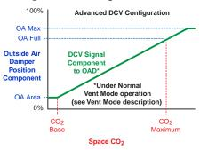
Although Advanced DCV is the most complex to configure, it is more energy efficient than Standard while still optimizing IAQ.
